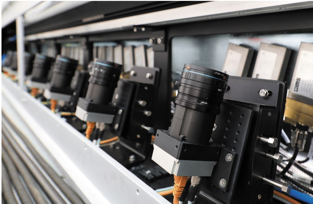
Figure 2 (Source IMS Messsysteme GmbH): 100% online inspection with high-performance LEDs and fast line scan cameras
