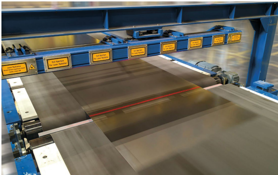
Figure 1: Intelligent cameras bundled into clusters guarantee highest measuring accuracy for flatness/evenness measurement even on high-gloss materials
