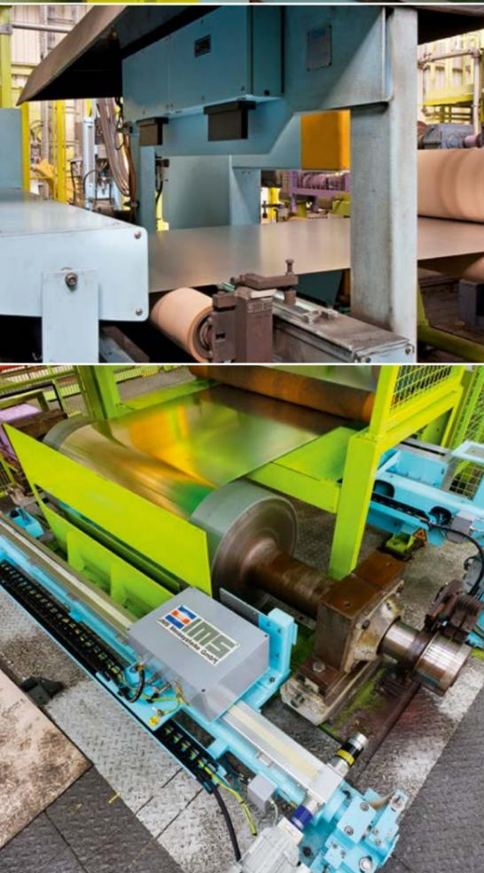
In finishing lines the input coils are first welded together to form a continuous strip. The loop tower ensures a continuous supply of strip material so that continuous strip pass through the tinning section is guaranteed even during downtimes.
