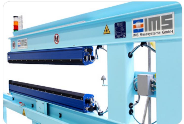
There are 50 image sensors in a beam-shaped camera housing per metre measurement range. The “mini-cameras” are lined up next to each other with a gap of 20 mm in between. The field of vision of the cameras used for evaluation of the data lies near their optical axes, which means the defects can be detected optimally.
