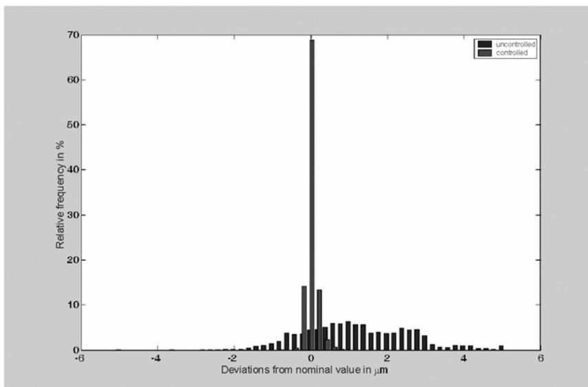
**Fig. 11. Typical distribution of paint coating thickness deviation – comparison between manual and automatic operating modes**
