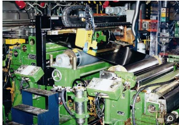
*Fig. 2. Paint coater – scanning gauge*
