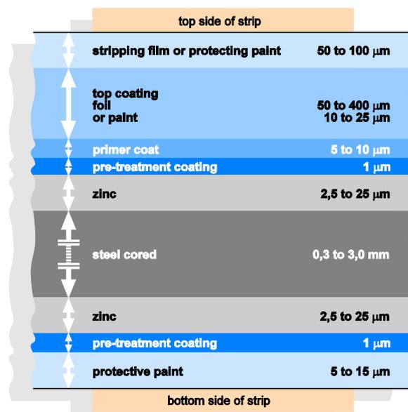
*Fig. 3. Schematic presentation of a layered paint coating on galvanised steel strip*
