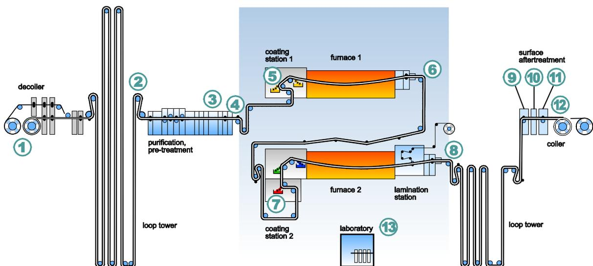
Fig. 1. Typical layout of a colour-coat line
