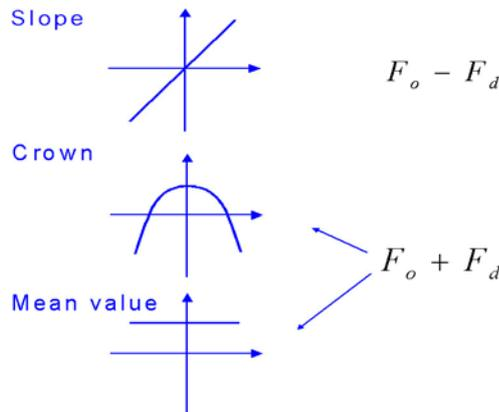
Fig. 6. Breakdown of paint profile into separate components
