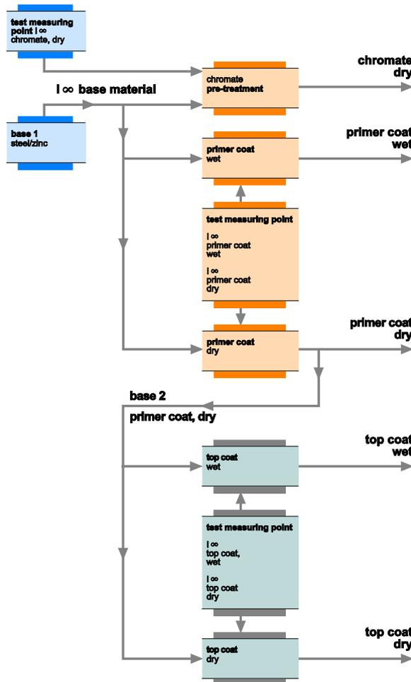
Fig. 4. Signal flow diagram – multi-layer measurement
