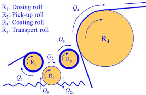
Fig. 5. Schematic presentation of a four-roll coater operating in reverse mode
