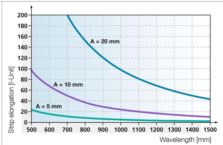
Flatness errors at a given wavelengths and different amplitudes A, typical strip elongation in hot strip applications
