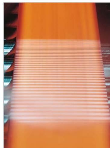
ity is determined using a test body of known shape. A dynamic method based on the shift in phase between the reference level and the test object is used to analyse the lines (phase-shift method).
